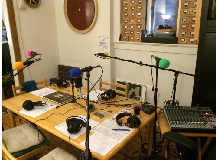
A round table would be even better, but we're able to arrange the mics so that cast members generally aren't sitting in the pickup pattern of each other's mics. We can also assign each cast member a specific spot in the stereo mix, through the pan controls on the mixing board. We make up for not having live Foley through heavier post, and we're fortunate to have good free sound and music resources available on the Internet.
